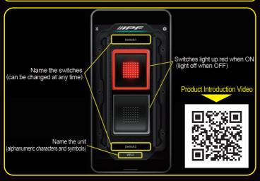
Control unit of the WR wireless switch incorporates two manual ON/OFF switche linked to IPF CONNECT app, allowing you to turn lights on and off in case your phone runs out of power.
