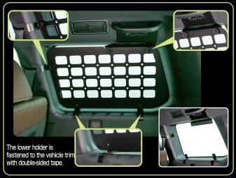
Easy installation without modifications on vehicle side, with 3-way (5-point) fastening for strong attachment.
