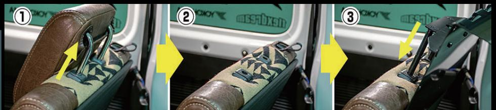
Easy installation with no modifications, by simply inserting it into the installation holes.
