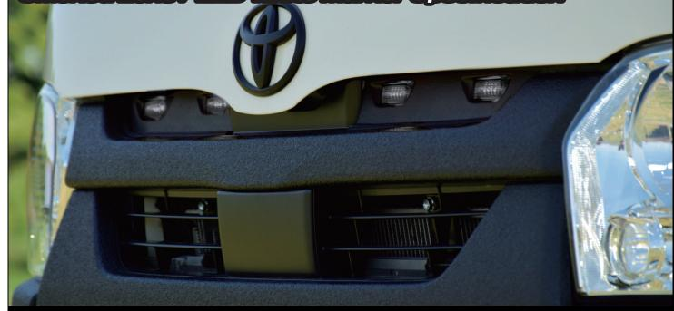
Smoked Lens/White Light Specification LED markers use vehicle inspection compliant units rated at 300 cd or below
