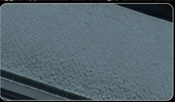
\*As it is made of urethane resin, it can be used unpainted; however, it will whiten and deteriorate over time, so we recommend painting it.
