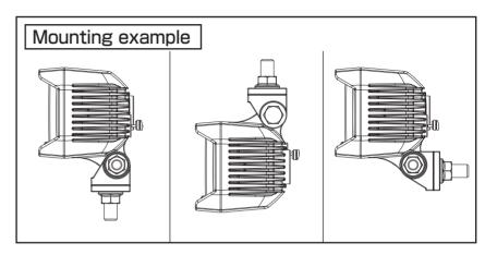
2. Using provided M10 nut and secure it on the vehicle's durable part.
