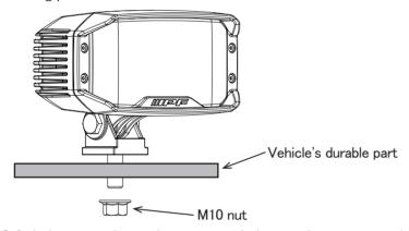
3. In below mounting option, unscrew bolts to orientate outer rim. IPF logo should be in a readable position.
