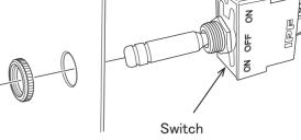
Remove the face nut from the switch and attach it from the front side. See the image above.
