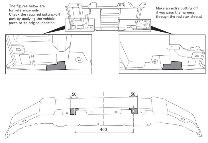
The above figure shows the layout of the JB64. JB74 has different configuration in some parts.
