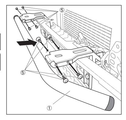
(4) Cut off the part of the radiator shroud and front bumper indicated below that interferes with the brackets.
