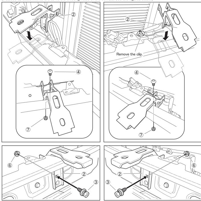
(3) Fix the bar (1) with the button bolts (5) tighten to the brackets 2 that were temporarily fixed to the vehicle in the process (2).
