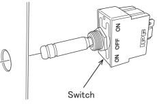
Remove the face nut from the switch and attach it from the front side. See the image above.
